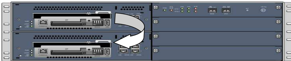
SV8500's showing connection points for hot Standby mode
