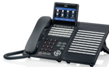
DT930 + 60-line DSS Console
